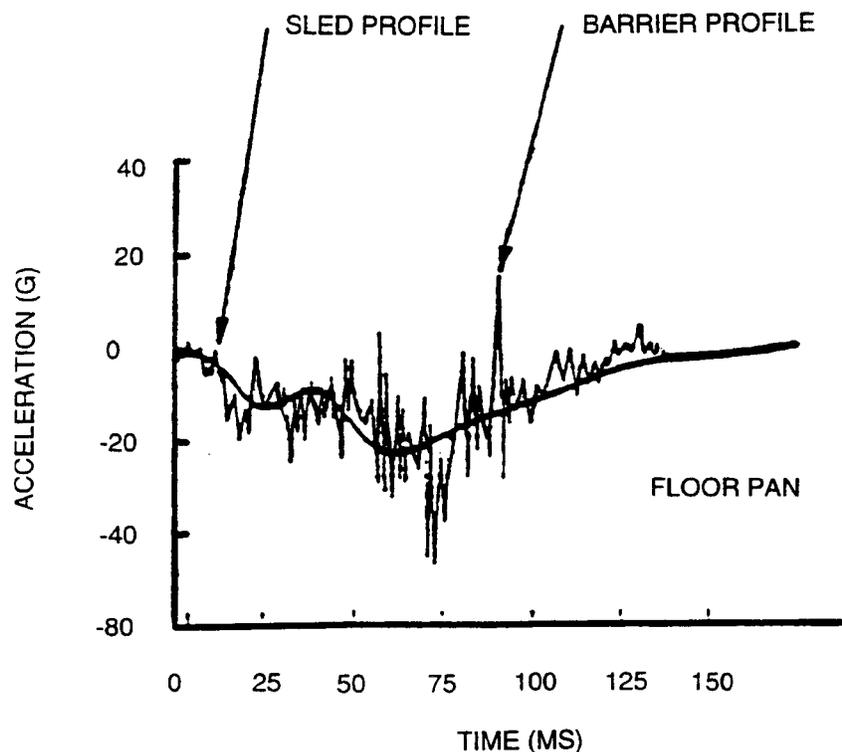
FIGURE 13—48 KM/H (30 MPH) BARRIER AND SLED SHOCK PROFILES
